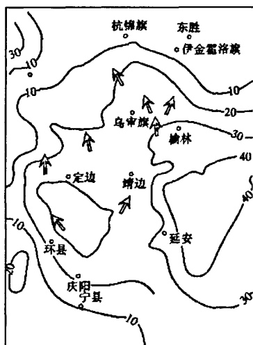
图1 鄂尔多斯盆地上古生界生气中心及油气运移方向示意图 Fig.1 Schematic map showing gas-generating centers and direction of oil-gas migration
