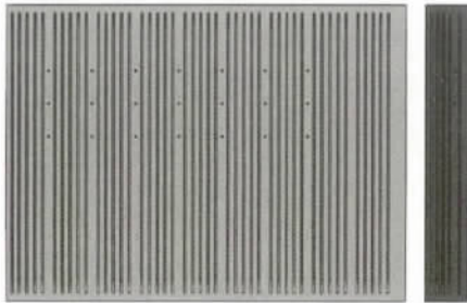
图2 铜板背面热电偶和水槽分布 Fig.2 Thermocouples and sinks distribution on the back
