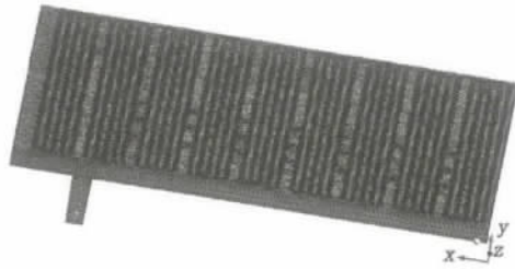
图1 1/4铜板三维有限元模型 Fig.1 The-dimensional finite element model of 1/4 copper plate
