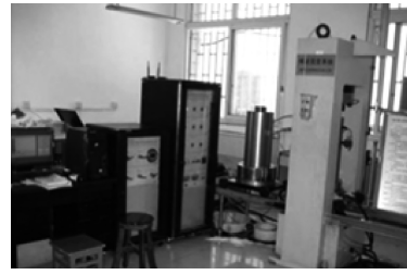
图5 岩石三轴流变试验系统 Fig.5 Triaxial rheological test system of rock
