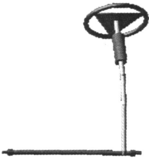
图2 齿轮齿条转向系统 Fig.2 Gear and rack steering system
