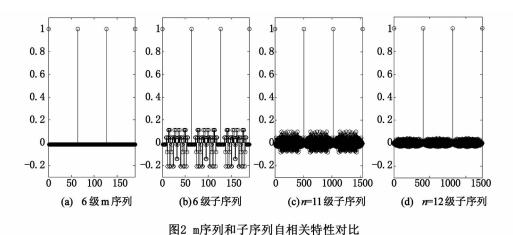
Fig. 2 Autocorrelation comparison for m sequence and its sub-sequence
