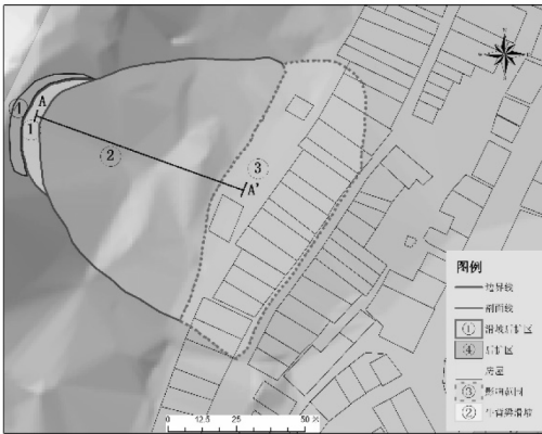
图 6 牛背梁滑坡及其影响范围 Fig.6 Niubeiliang landslide and its impact range
