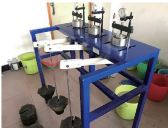
图 1 普通高压固结仪 TKA-STC-3H Fig.1 Ordinary high pressure Consolidator TKA-STC-3H
